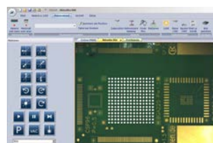
Superimposing of component and target position
