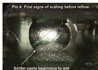
PBGA – scaling: insufficient heat
