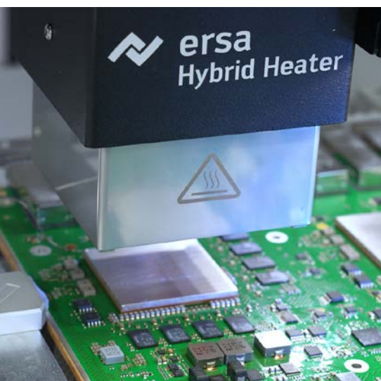
Hybrid heating head while desoldering a metallic BGA
