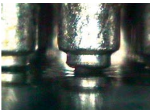
CCGA: insufficient solder
