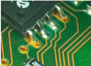
Lead-free assembly: non-wetting
