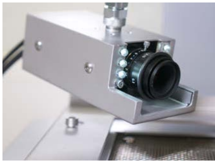
Reflow Process Camera (RPC) on the HR 550
